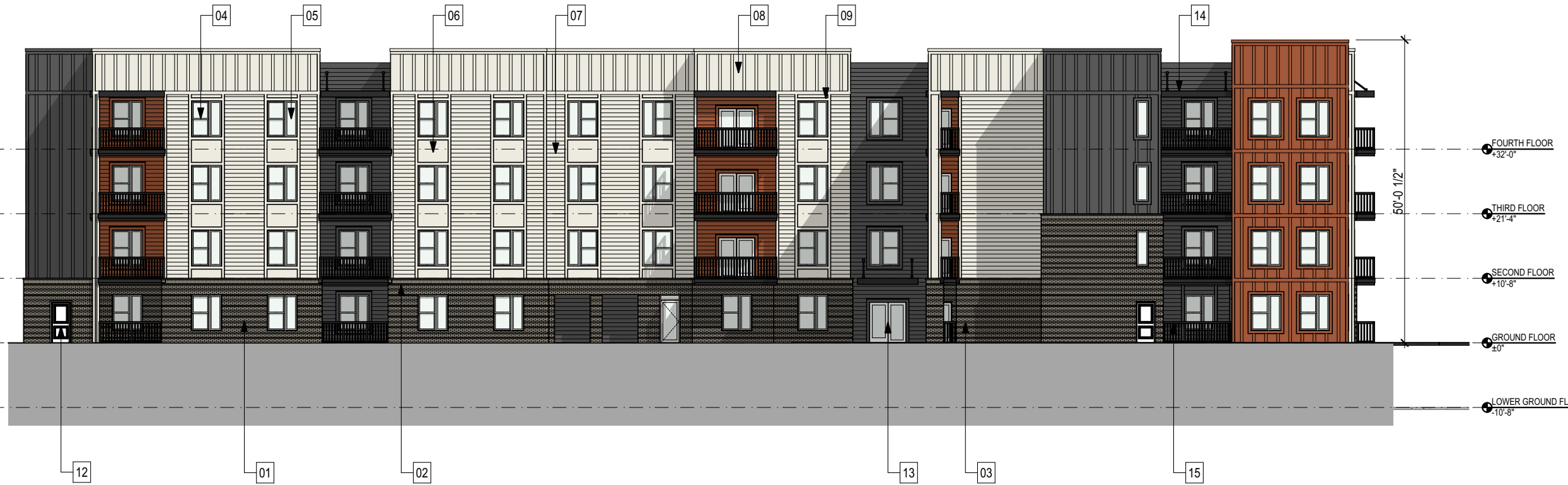
BUILDING A NORTH ELEVATION
