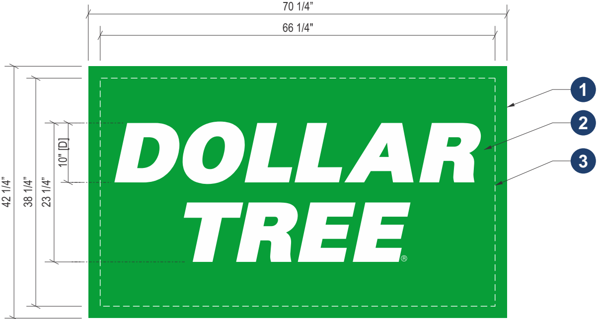
Panel Replacement On Existing D/F Pylon QTY 2 (1 SET)
