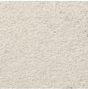
SS2 SYNTHETIC STUCCO AT TRIM/DETAILS SAND FINISH
